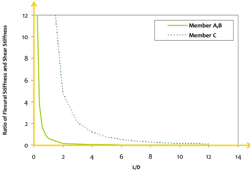
Figure 3.32: Role of Relative Translational Stiffness: Influence of  $L/D$  ratio on  $\beta$  of frame members
