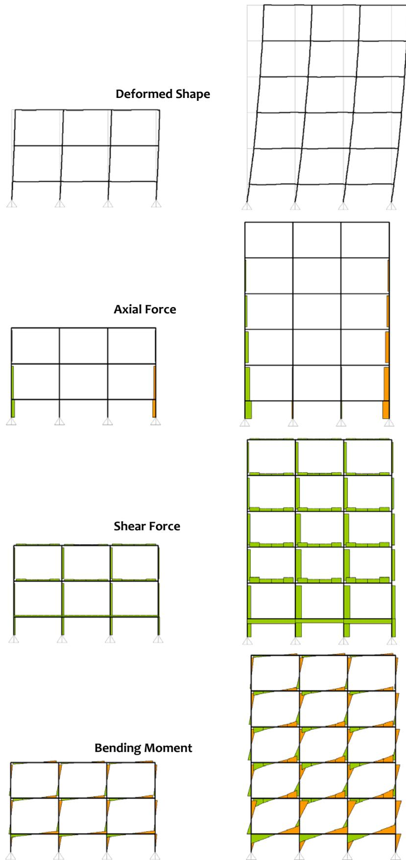
**Figure 3.104:** Buildings with *Step-back*: Deformation and force distribution
