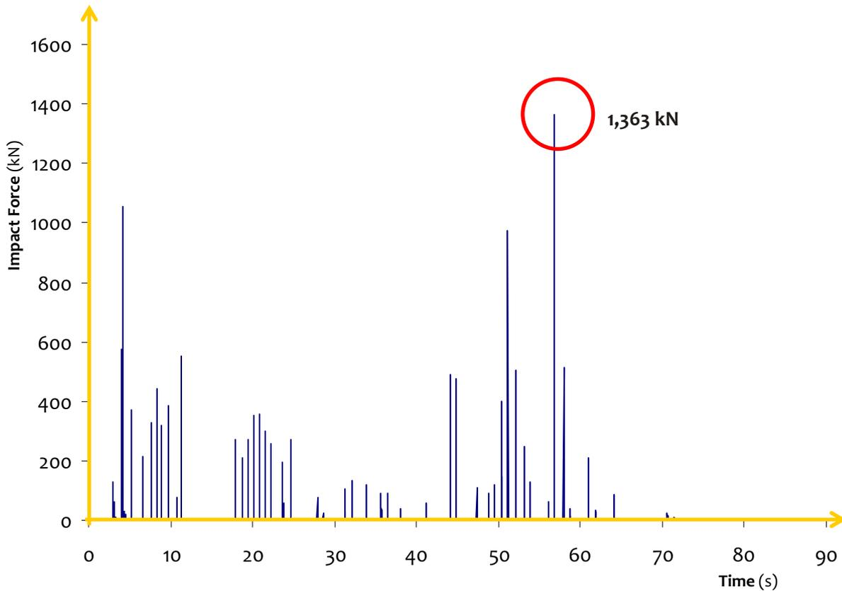
**Figure 4.75:** *Pounding of adjoining buildings:* Time history of impact force at one on the roof level of the buildings - (a) two identical 5-storey benchmark buildings, (b) 5-storey benchmark building and another 4-storey building, and (c) one 5-storey benchmark building and one 10-storey building.
