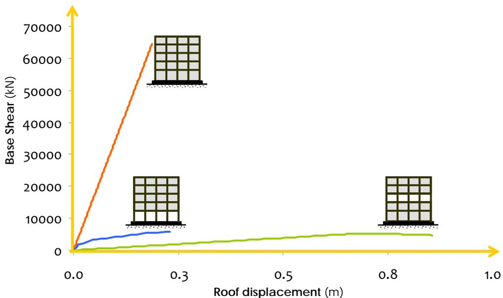
**Figure 4.31:** *Discontinuing Structural Walls in a building: It creates a weak link in the building's lateral load resisting system, and severely incapacitates the building from resisting the lateral shaking in spite of the presence of Structural Walls in the other storeys*
