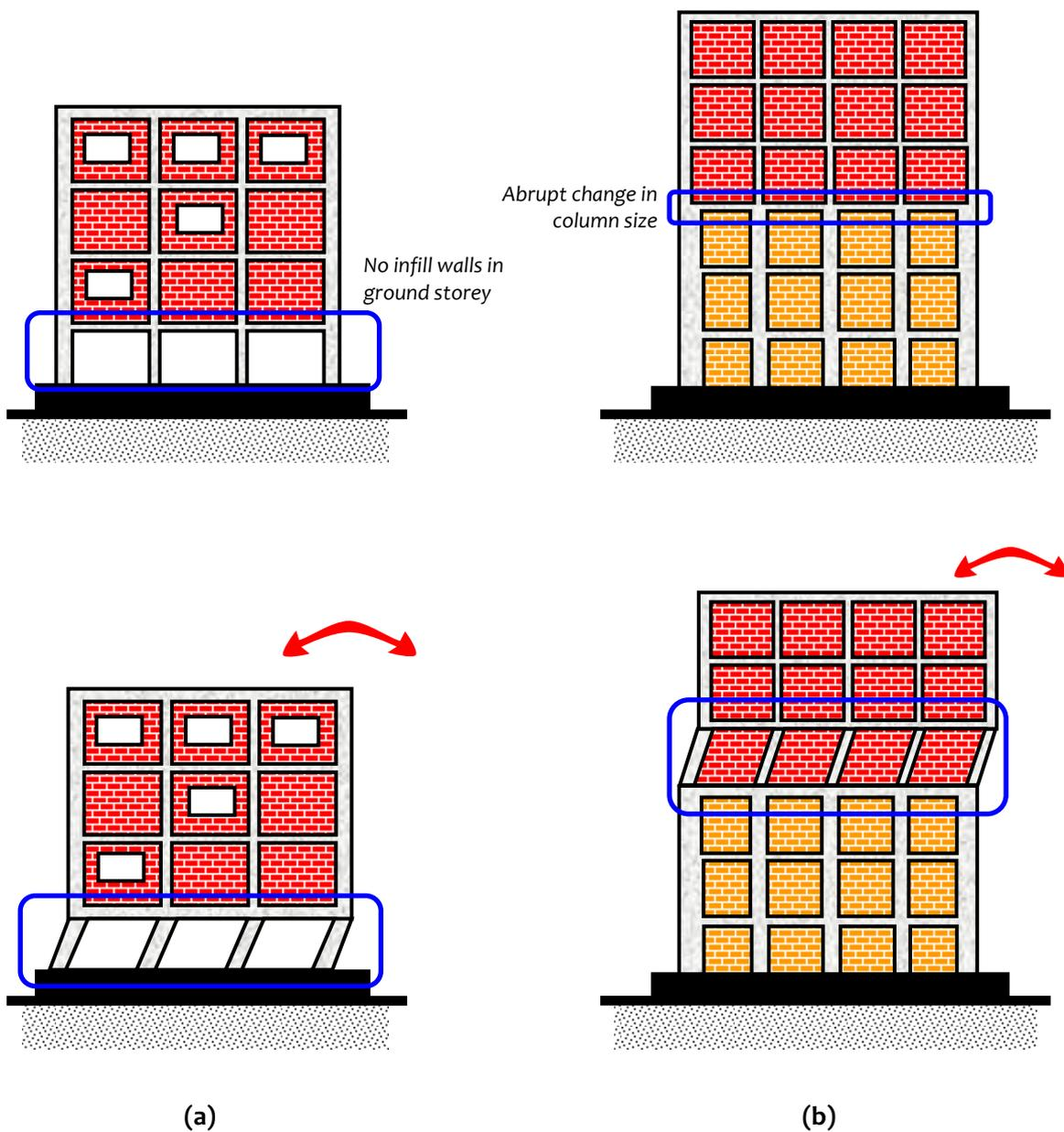
**Figure 4.22:** Lateral strength discontinuity or reduction of lateral strength along height of building: Strength reduction affects inertia force transfer – (a) open storey, and (b) change in member sizes
