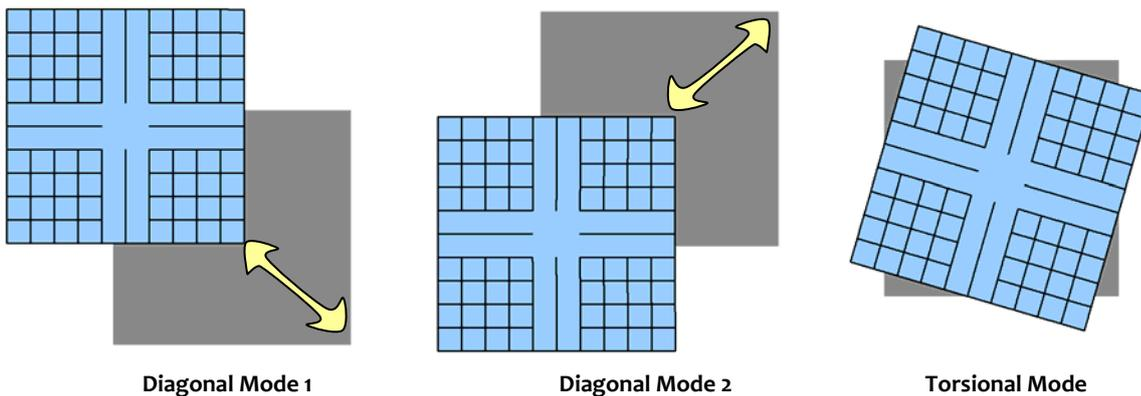
**Figure 2.17:** Diagonal modes of oscillation: First three modes of oscillation of a building symmetric in both directions in plan; first and second are diagonal translational modes and third rotational
