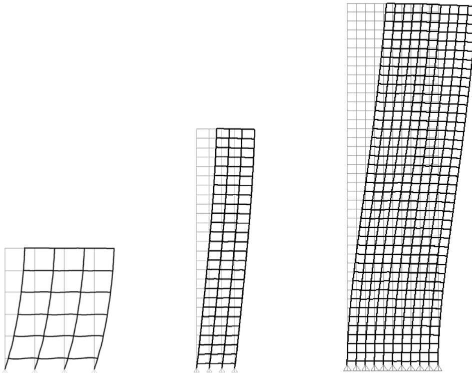
**Figure 2.22:** *Effect of building height:* Fundamental translational mode shape of oscillation does not change significantly with increase in building height, unlike the fundamental translational natural period, which does change
