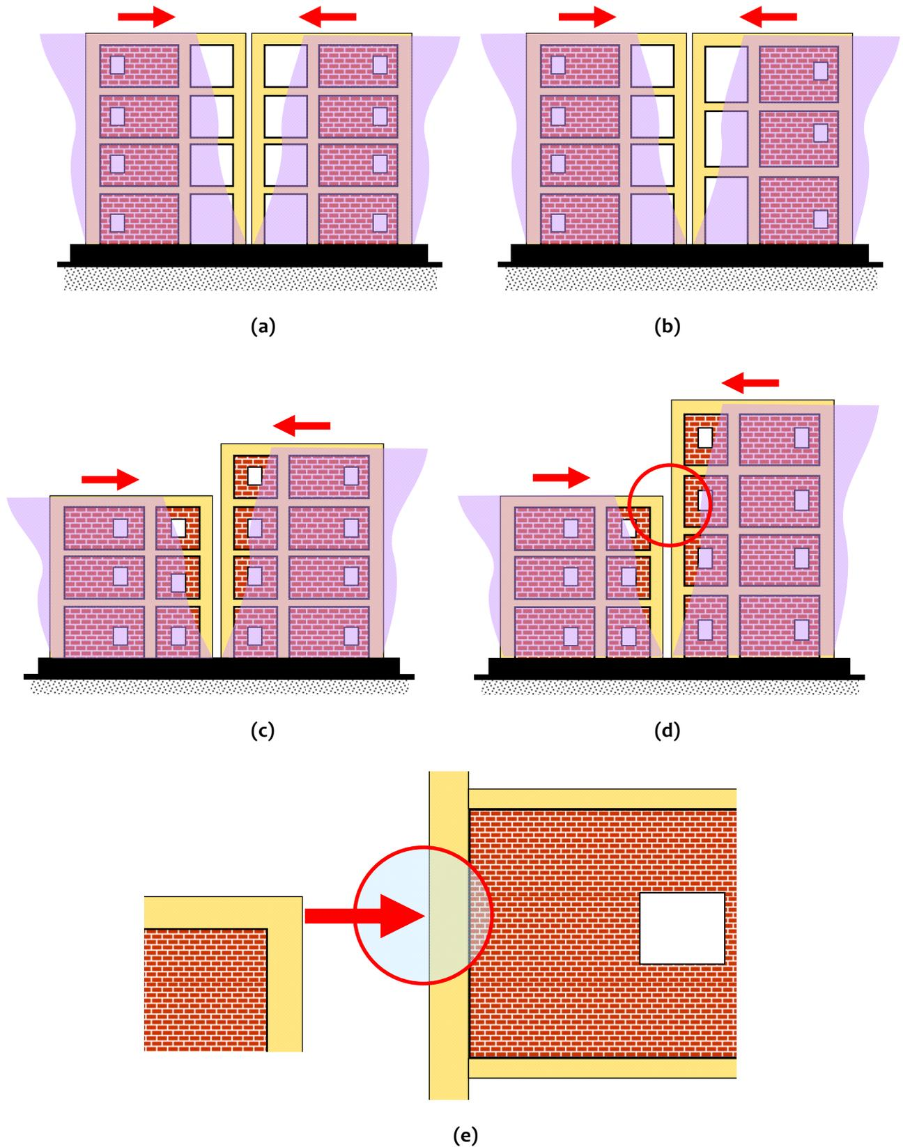
**Figure 3.107:** *Pounding within a building with expansion joints:* Four possible configurations of buildings - (a) two parts with same overall height and same floor heights, (b) two parts with same overall height and different floor heights, (c) two parts with different overall height and same floor heights, (d) two parts with different overall height and different floor heights, and (e) local action of a floor on the column of the adjoining (part of the) building
