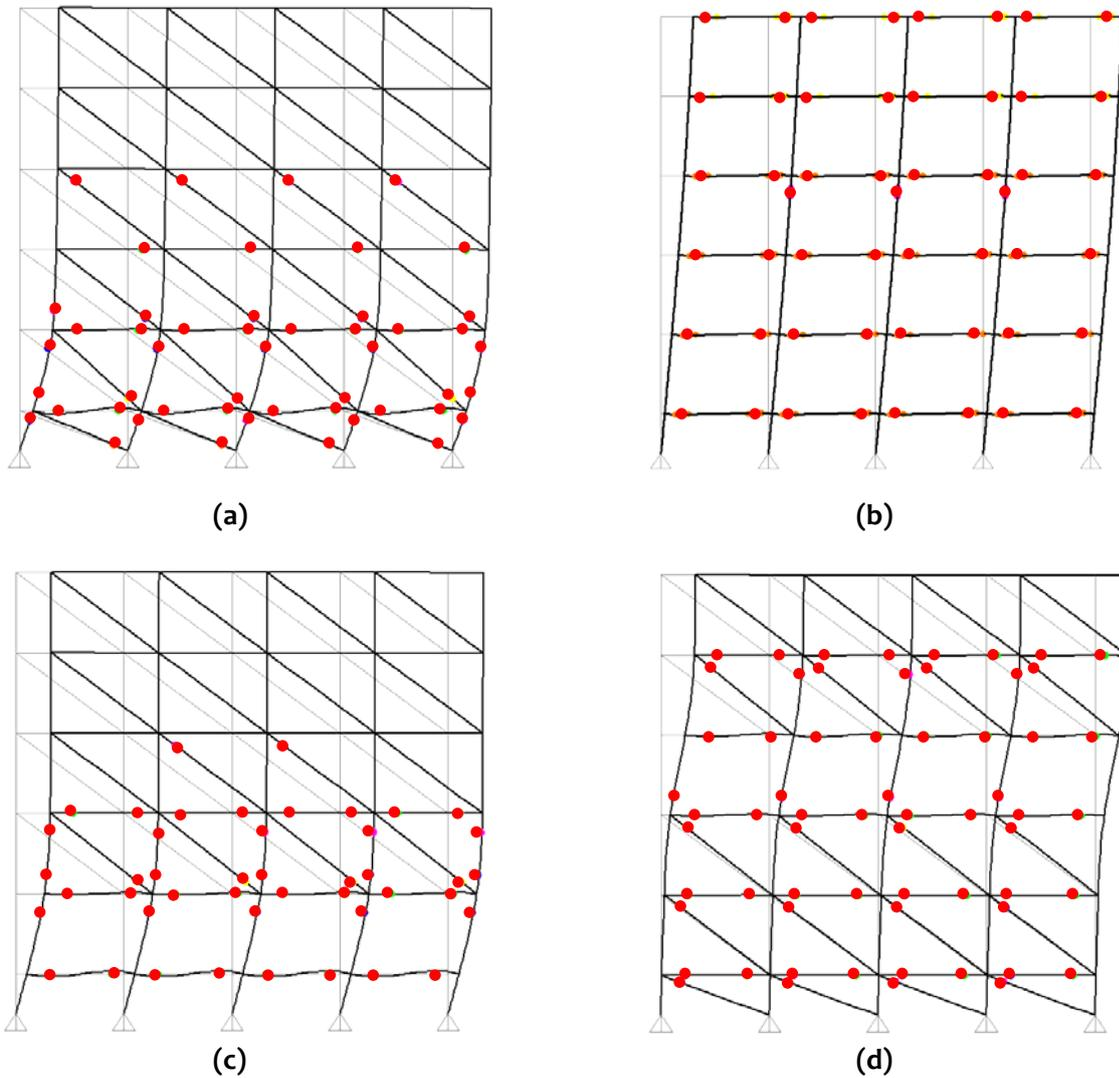
**Figure 4.28:** *Open storey in a building:* Deformation is uniform when the building has no sudden discontinuity (as in (a) and (b)), but all lateral deformation in building concentrated in open (flexible and weak) storey in building without infills (as in (c) and (d))
