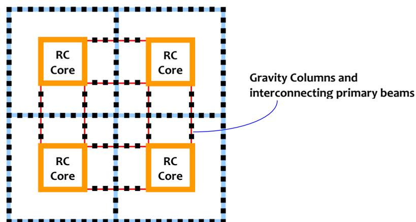
**Figure 3.61:** *Connection between RC Cores in a Bundled-Tubes System:* Gravity columns and interconnecting primary beams form the link between the stiff and strong RC cores inside the tubes
