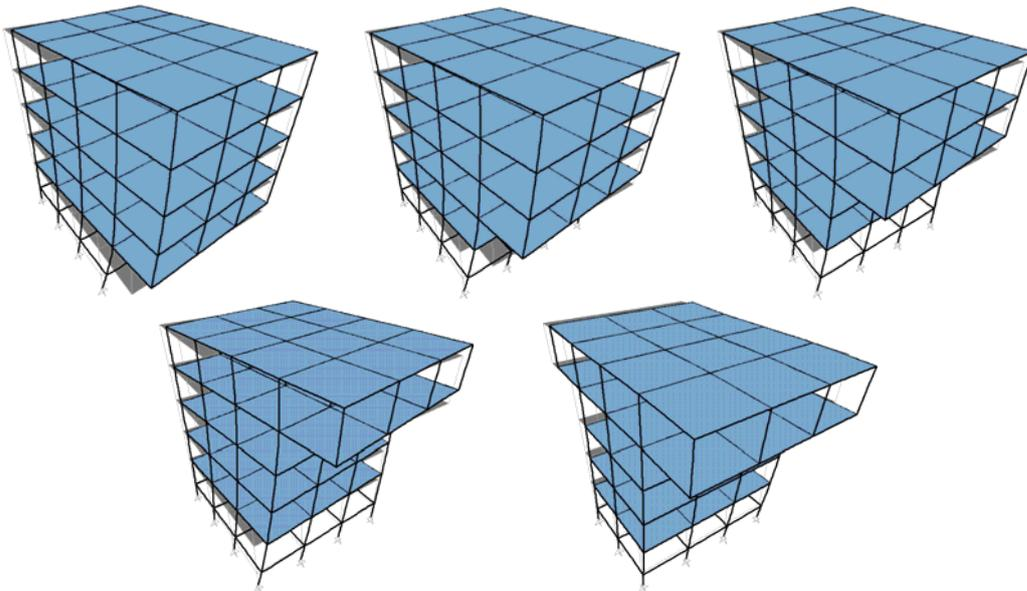
**Figure 3.102:** *Fundamental modes shapes of buildings with vertical irregularity in overall geometry:
