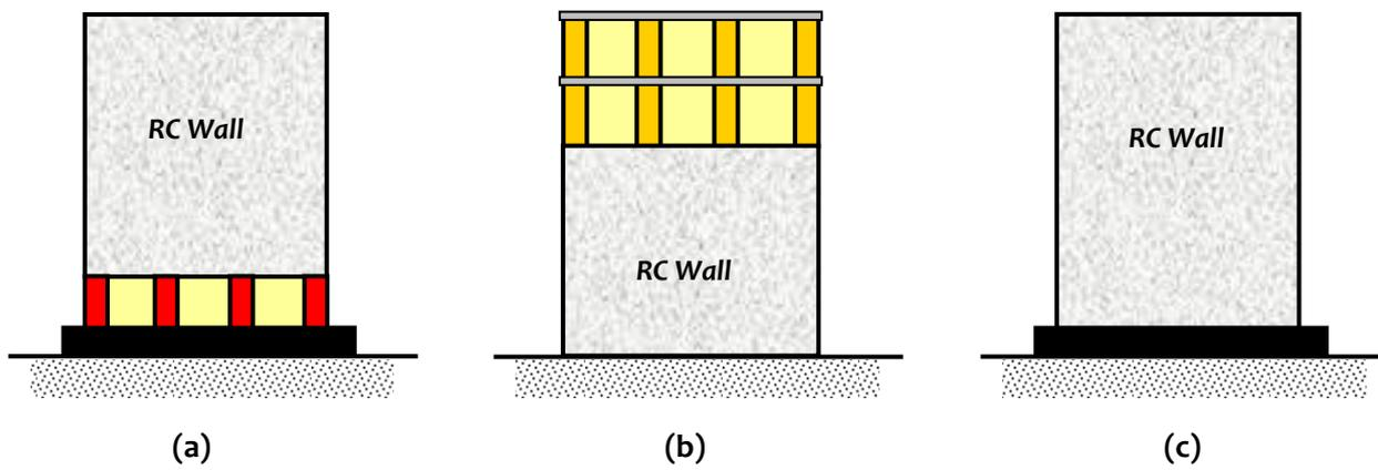
**Figure 4.29:** *Discontinuing Structural Walls in a building:* (a) Structural wall discontinued in ground storey, the worst choice, (b) Structural wall discontinued in upper storeys, also an unacceptable choice, and (c) Structural wall not discontinued, the best and *only* option
