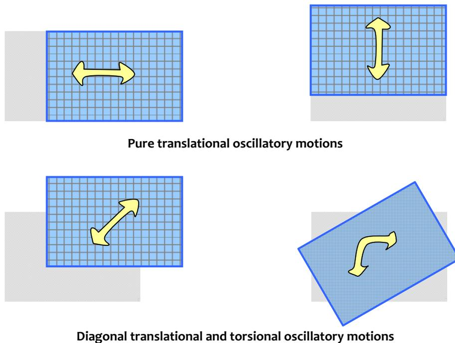
**Figure 3.3:** Oscillatory motions of buildings during earthquake shaking: Diagonal translational and torsional oscillations are not preferred
