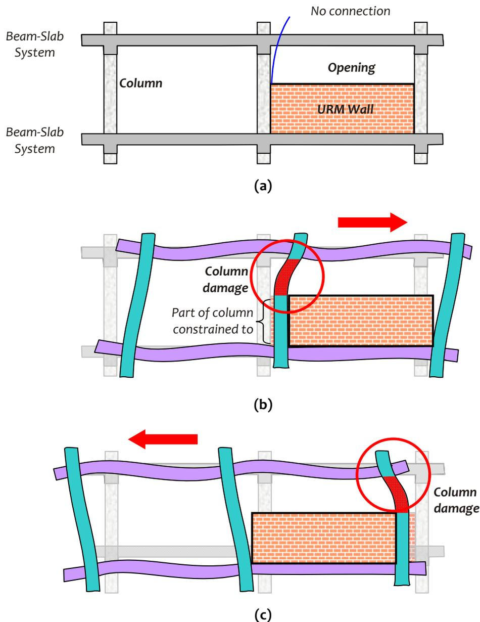
**Figure 4.33:** Short column effect owing to masonry infills adjoining the RC columns in buildings: Effective height of column over which it can bend is restricted by adjacent walls; this short-column effect is more severe when opening heights are small
