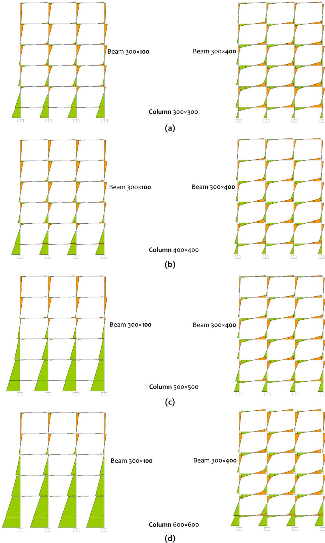
**Figure 3.41:** Bending moment in members of benchmark building subjected to lateral load with different combinations of beams and columns: Bending moment increases in column with reduction in beam-to-column flexural stiffness
