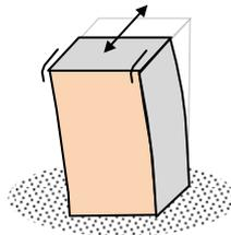
**Building with NO Lateral Load Resisting System ( Building A1)**
