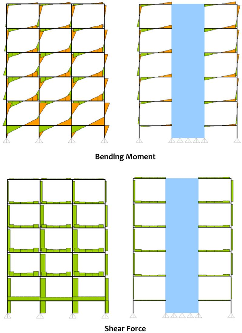
**Figure 3.43:** Building with structural walls at periphery: Demands on beams and columns are significantly reduced in buildings with structural wall
