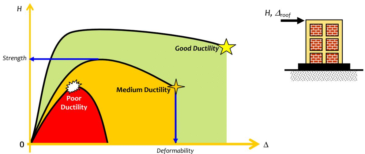
**Figure 1.6:** *Ductility*: Buildings are designed and detailed to develop favorable failure mechanisms that possess specified lateral strength, reasonable stiffness and, above all, good post-yield deformability.
