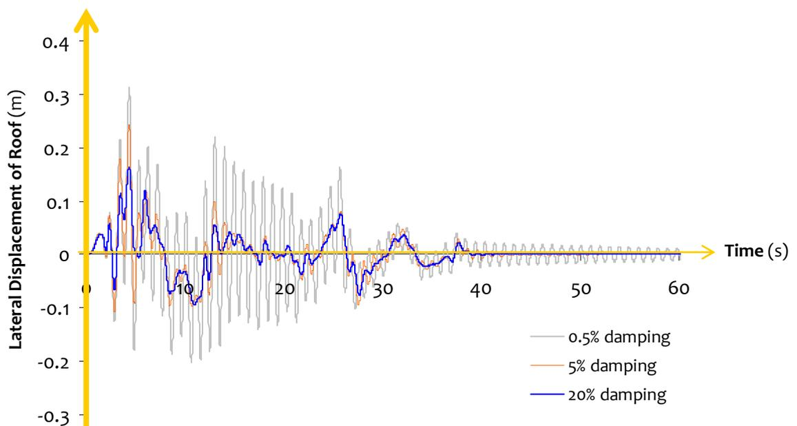
**Figure 2.29:** *Effect of damping:* Amplitude of oscillation reduces with increase in damping
