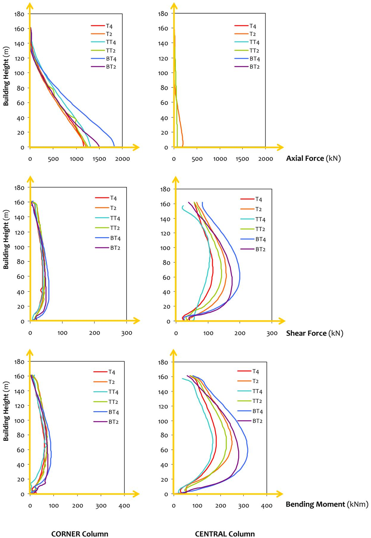
**Figure 3.65:** Variation of forces in Columns in the Tube (2m column spacing) along height of building: Force transfer in the lower storeys takes place largely through axial action in corner columns
