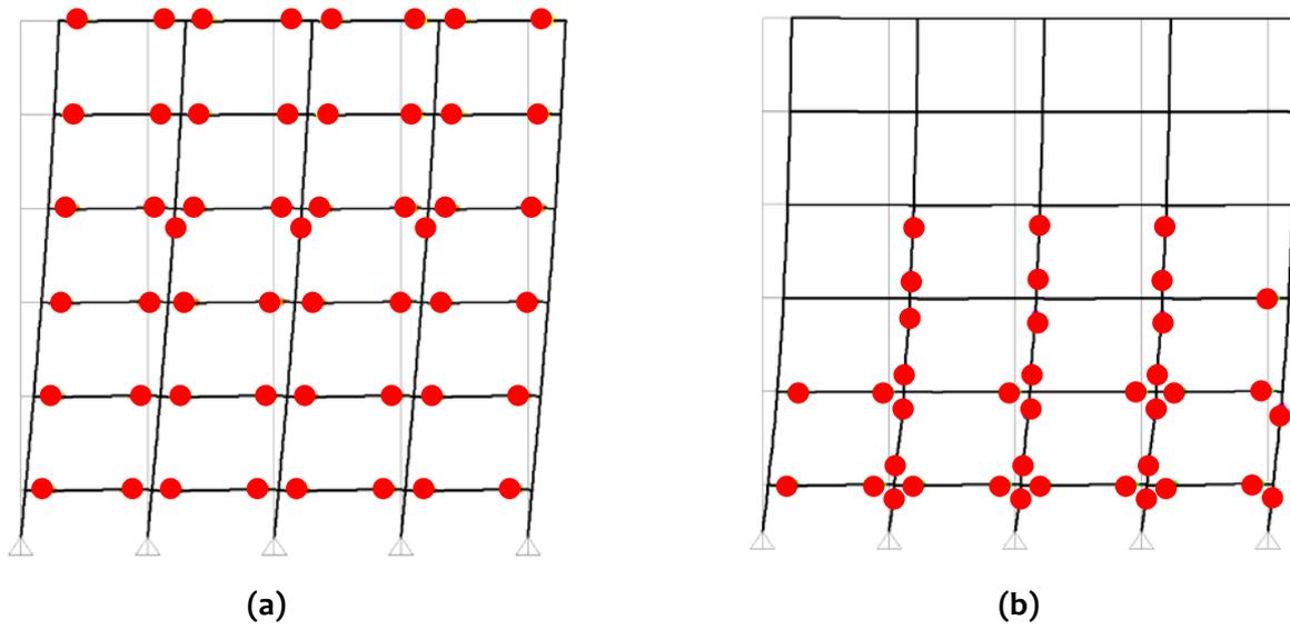
**Figure 4.7:** *Strength hierarchy of frame members:* Columns sustain large plastic actions when design of building follows WC-SB concept - (a) Strong column - weak beam (SC-WB) design, and (b) Weak column - strong beam (WC-SB) design
