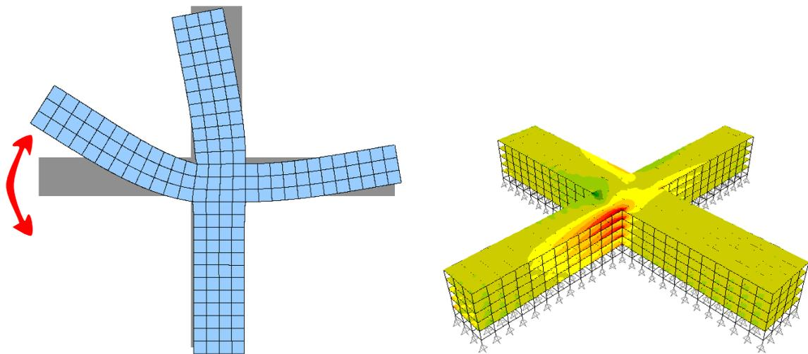
**Figure 3.15:** *Dog-tail-wagging mode of oscillation:* Dog-tail-wagging mode of oscillation in building with X-plan shape cause significant stress concentration at re-entrant corners
