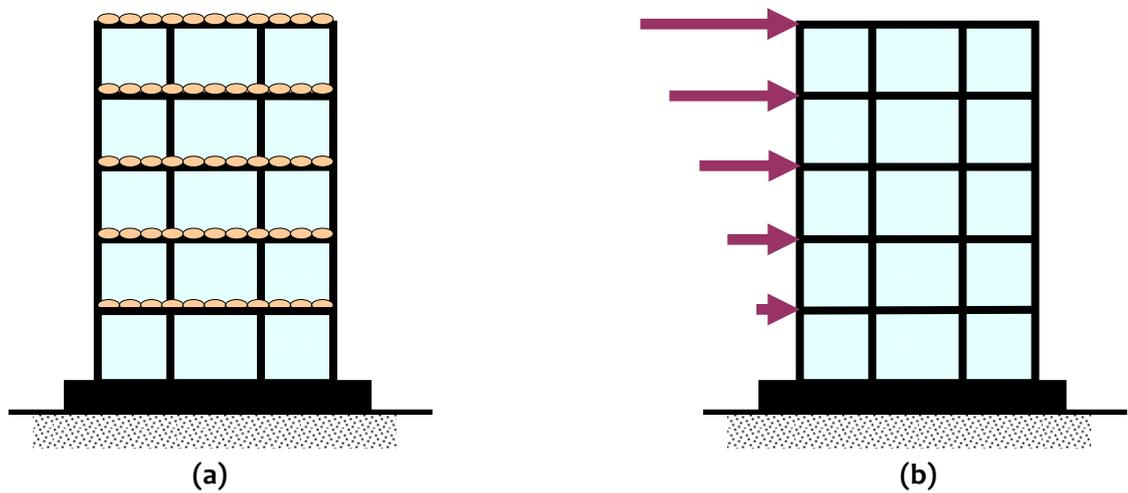
**Figure 3.37:** Two basic load types on moment frames: (a) *Gravity Loads*, and (b) *Lateral Loads*
