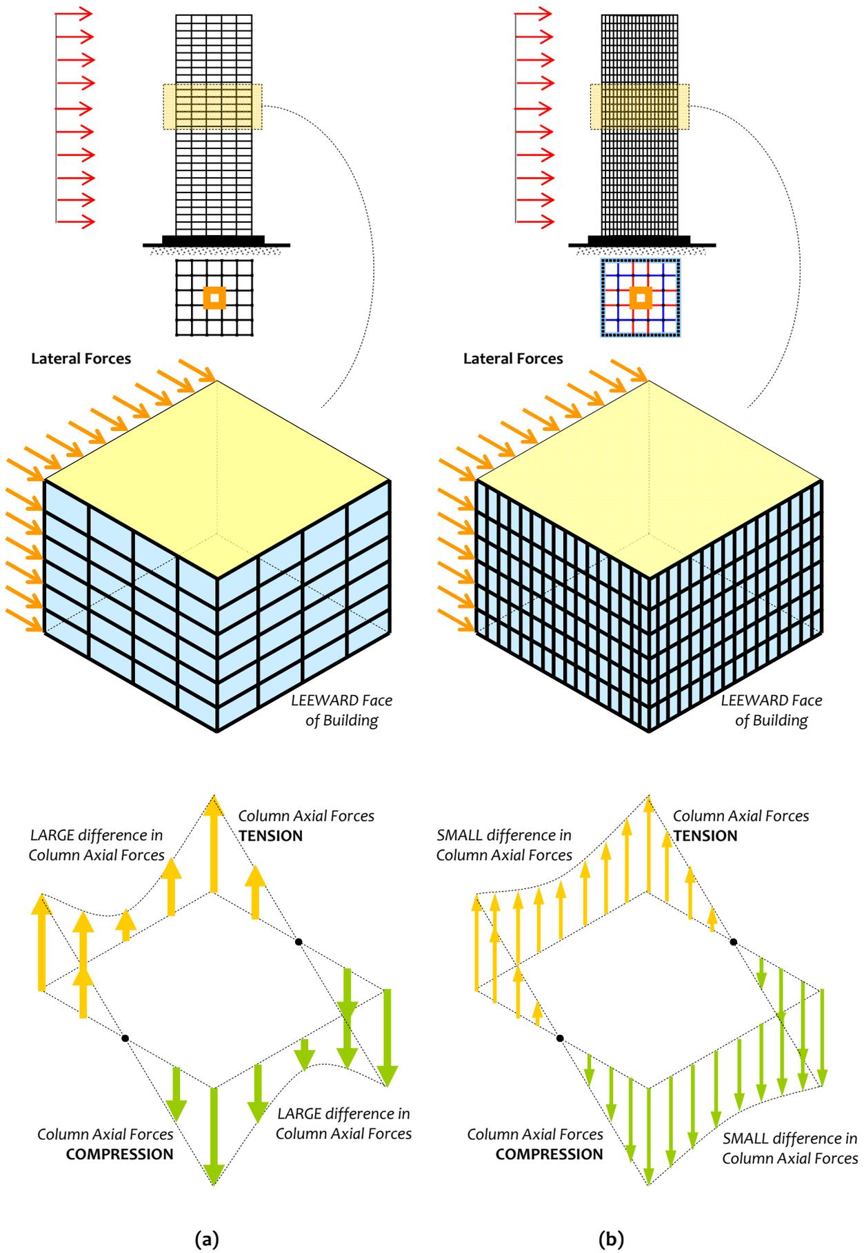
**Figure 3.57:** Shear Lag Effect in Structural Systems: (a) Traditional Frame System has large difference in column axial forces on leeward and windward faces, and (b) Tube System has small difference in column axial forces on leeward and windward faces
