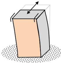
**Building with NO Lateral Load Resisting System ( Building B1)**
