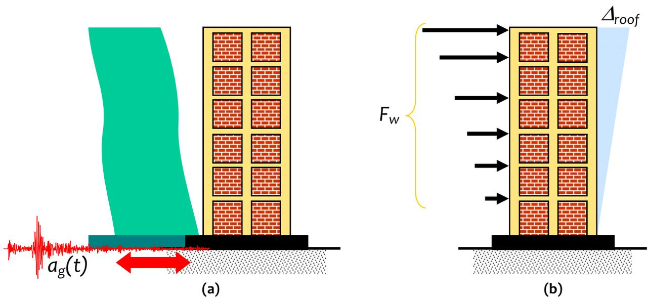
**Figure 1.1:** Difference in the design effects on a building during natural actions of (a) Earthquake Ground Movement at base, and (b) Wind Pressure on exposed area
