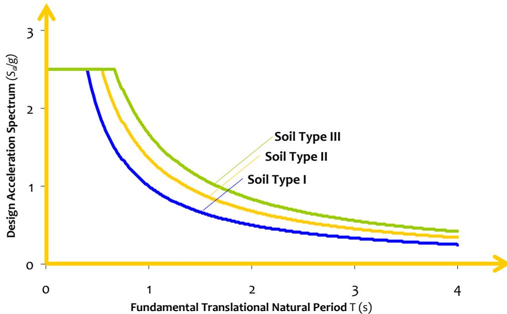
**Figure 2.2:** *Design Acceleration Spectrum:* This is based on fundamental translational natural period  $T$  of the building; this is defined in the following
