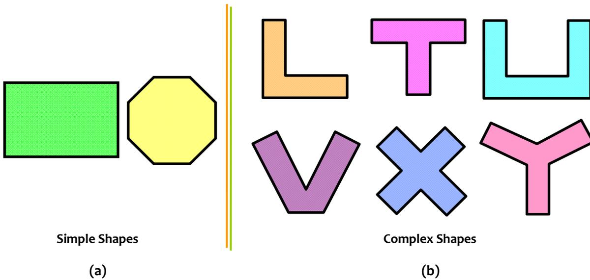
**Figure 3.1:** *Plan shapes of buildings:* Buildings with (a) simple shapes undergo simple acceptable structural seismic behaviour, while (b) those with complex shapes undergo complex unacceptable structural seismic behaviour
