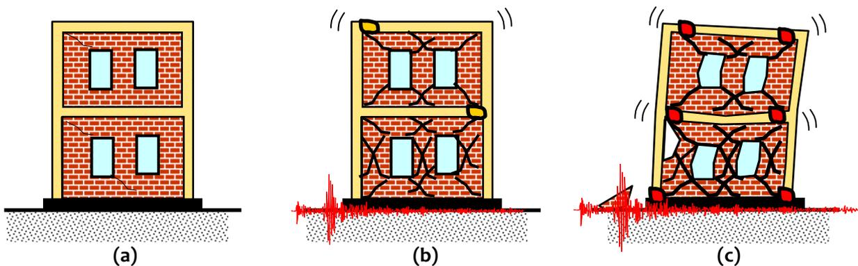
**Figure 1.3:** Earthquake-Resistant Design Philosophy for buildings: (a) Minor (Frequent) Shaking – No/Hardly any damage, (b) Moderate Shaking – Minor structural damage, and some non-structural damage, and (c) Severe (Infrequent) Shaking – Structural damage, but NO collapse
