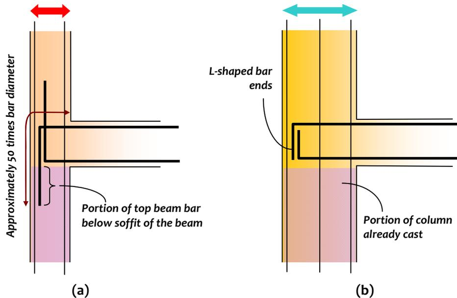
**Figure 4.13:** *Beam-Column Joints in Buildings:* Anchorage of beam bars in exterior joints: diagrams show elevation of joint region - (a) poor practice, and (b) good practice
