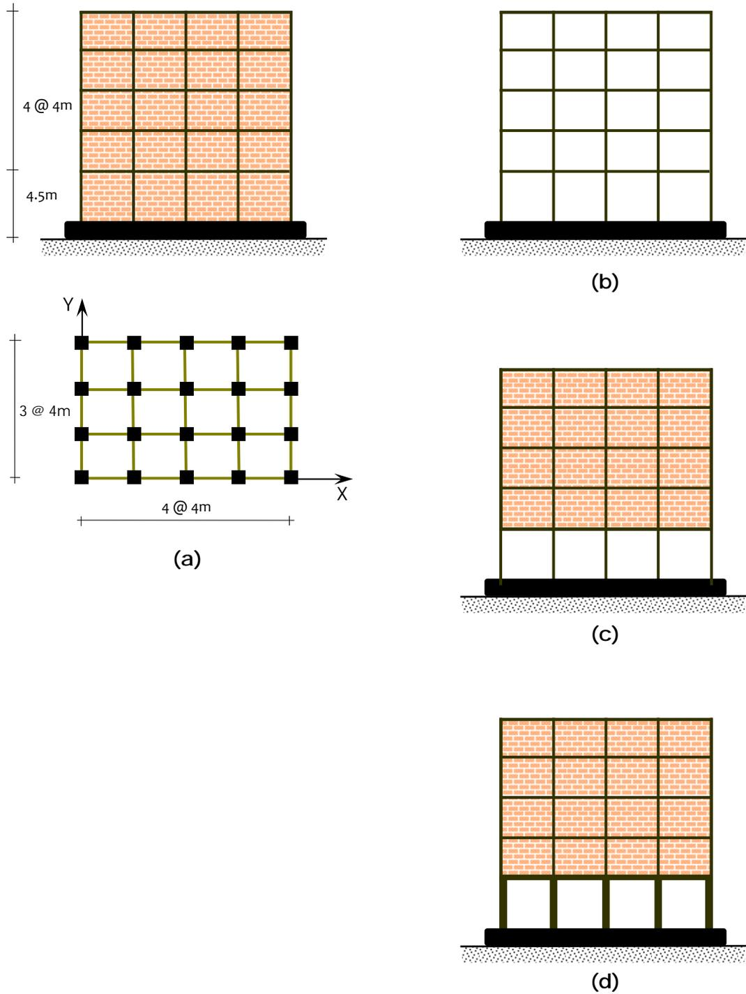
**Figure 4.66:** Open Ground Storey Buildings: Benchmark 5-storey building with (a) infills in all storeys, (b) with no infill masonry in any storey, (c) infill masonry in upper four storeys only, and (d) infill masonry in upper four storeys only and enhanced member designs in ground storey
