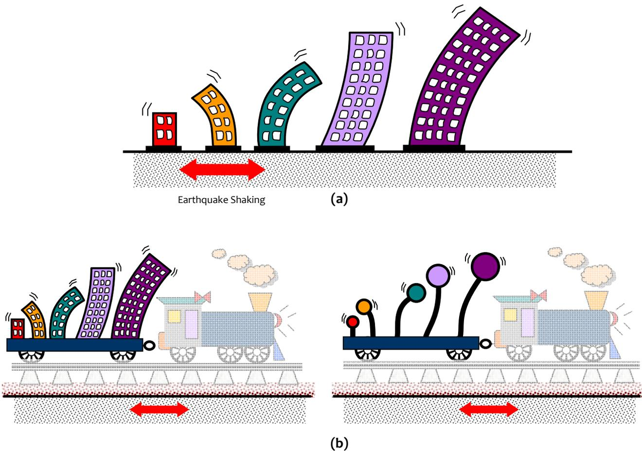
**Figure 2.34:** *Dependence of Response on Natural Period:* Time history of acceleration and displacement of mass is same for a number of structures with same natural period when subjected to the same earthquake shaking, and with same damping.
