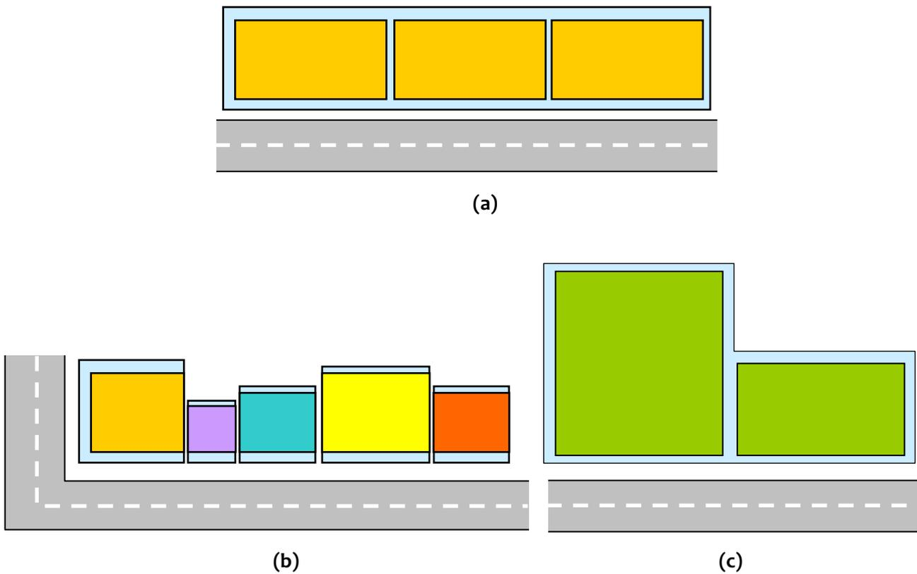
**Figure 3.106:** Building plan configurations that lead to two buildings / parts of building that pound on each other: (a) long building split in parts, (b) row construction, and (c) L-shaped building made in two parts
