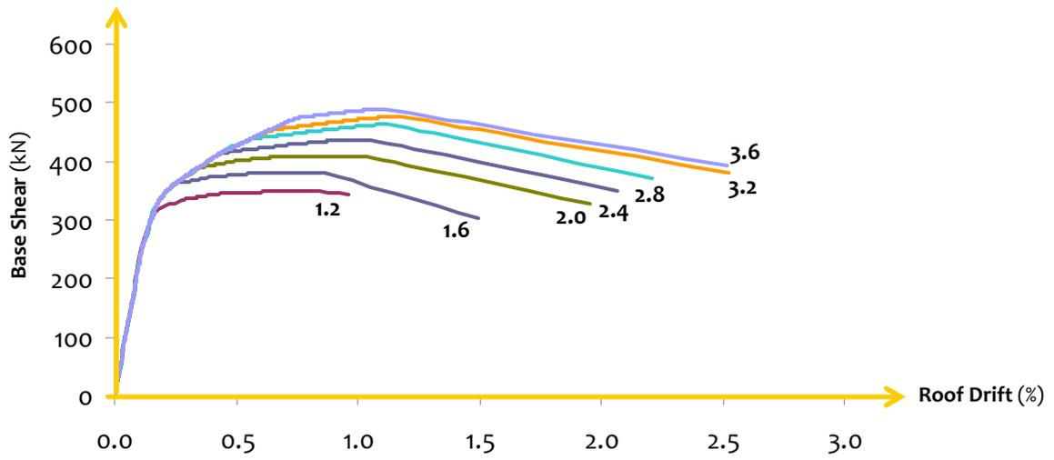
**Figure 4.69:** Capacity curves: Global ductility increases with increase in column to beam strength ratio in moment frames
