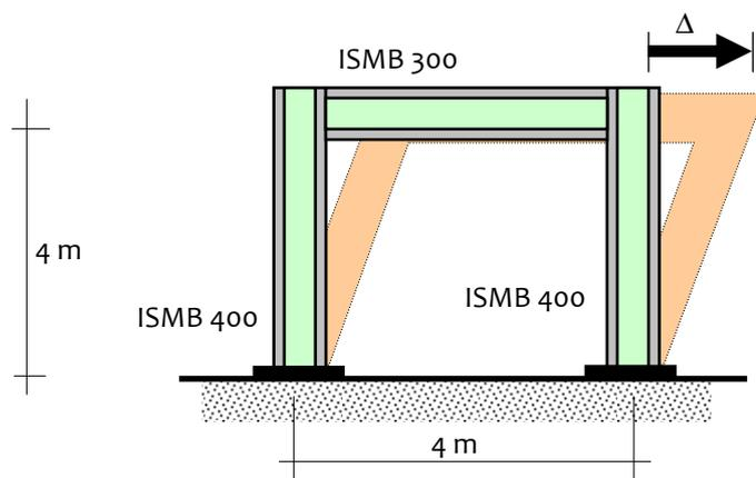
Figure 4.51: Portal frame considered to demonstrate ductility
