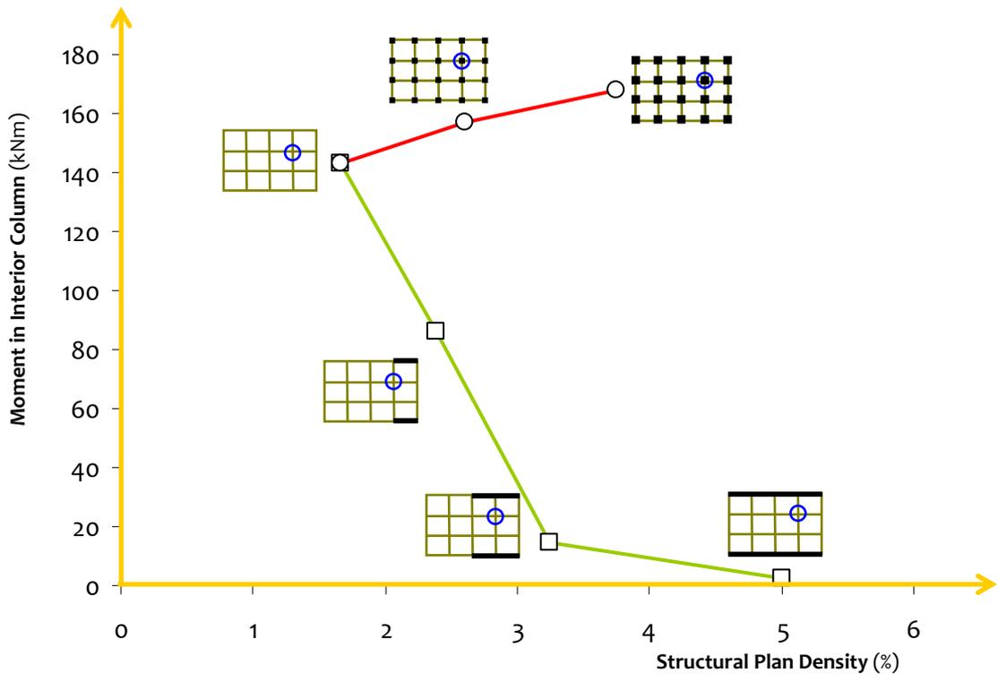
**Figure 4.17:** Structural Plan Density of vertical members in buildings: For the same area of vertical members (SPD), buildings tend to be more economic when structural walls are used, as against when columns of larger cross-sectional areas are used
