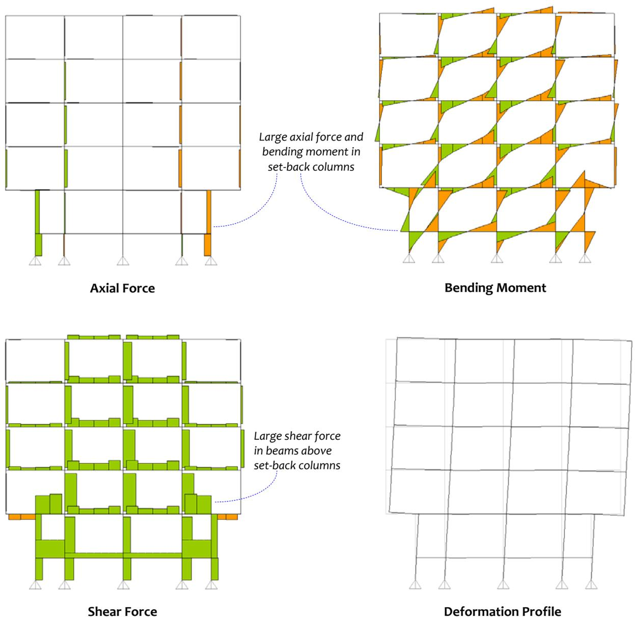
**Figure 3.73:** Buildings with set-back columns: Shear failure of beams above set-back columns is likely along with combined axial-flexural failure of set-back columns
