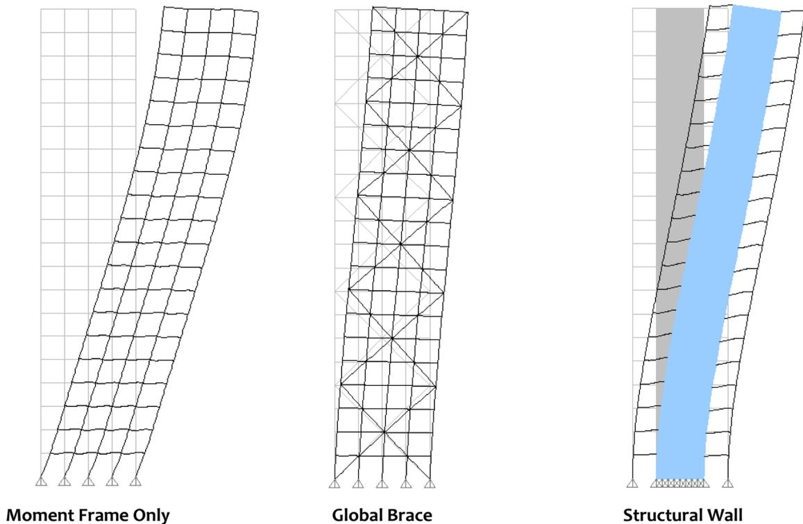
**Figure 3.52:** DEFORMATION PROFILES in buildings with no braces, global braces and structural wall: Lateral displacement is least in building with global braces, while it is maximum in (bare) moment frame buildings
