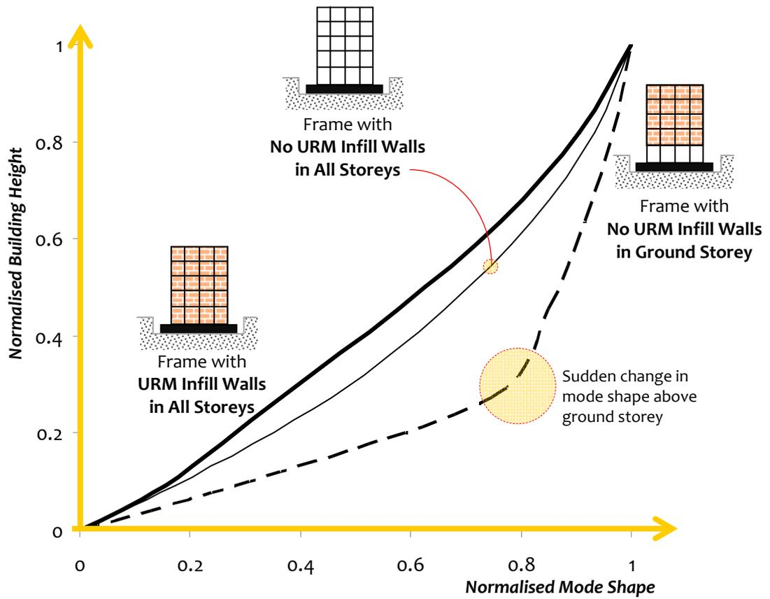
**Figure 2.27:** Influence of URM Infill Walls in Mode Shape of RC frame Buildings – Mode shape of a building obtained considering stiffness contribution of URM is significantly different from that obtained without considering the same
