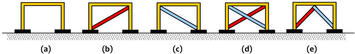
**Figure 4.56:** Frames considered in understanding implications of ductility on overall inelastic behaviour – (a) Bare frame, (b) Frame with tension brace, (c) Frame with compression brace, (d) Frame with diagonal X bracing, and (e) Frame with Chevron (inverted V) bracing
