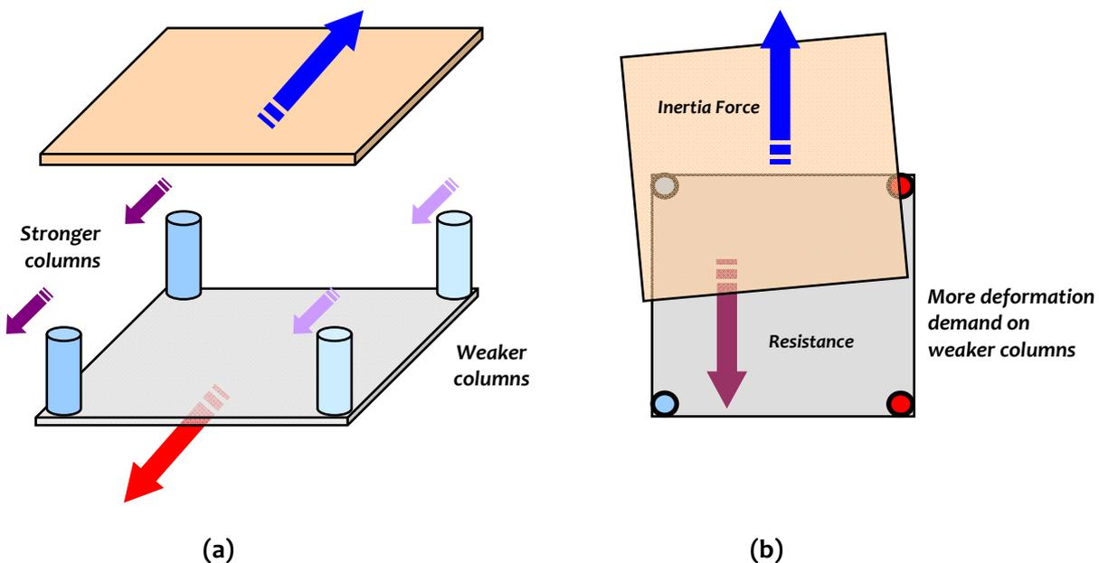
**Figure 4.18:** Lateral strength asymmetry in plan of a building: Lateral load resisting elements are critical in controlling earthquake behaviour of buildings – (a) four-column building has no stiffness and mass asymmetry so long as the behaviour is purely elastic, but (b) develops stiffness asymmetry at the onset of inelasticity in the weaker members
