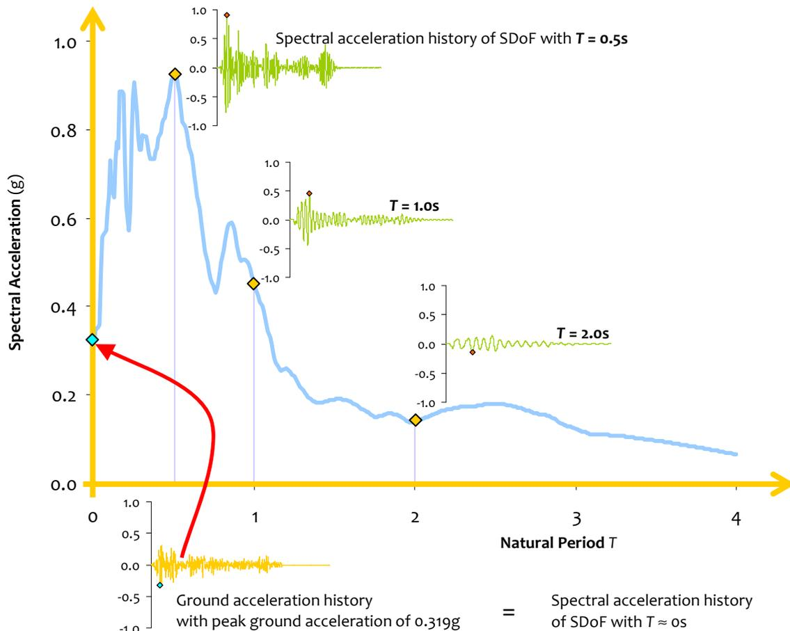
**Figure 2.36:** Acceleration Response Spectrum of a ground motion: Absolute maximum acceleration (or spectral acceleration) response of a spectrum of structures with different fundamental translational natural periods, but with the same damping and subjected to the same considered ground motion
