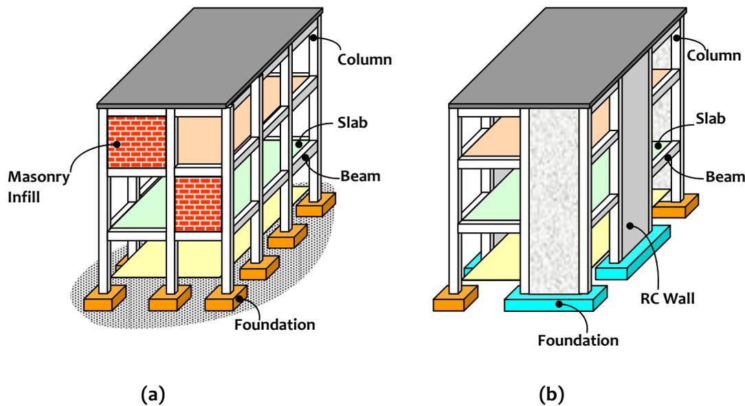
**Figure 4.15:** Use of Structural Walls in buildings: Walls of full-height provide a reasonably uniform stiffness and strength along the height: (a) Moment-frame building, and (b) Moment-frame building with Structural Walls
