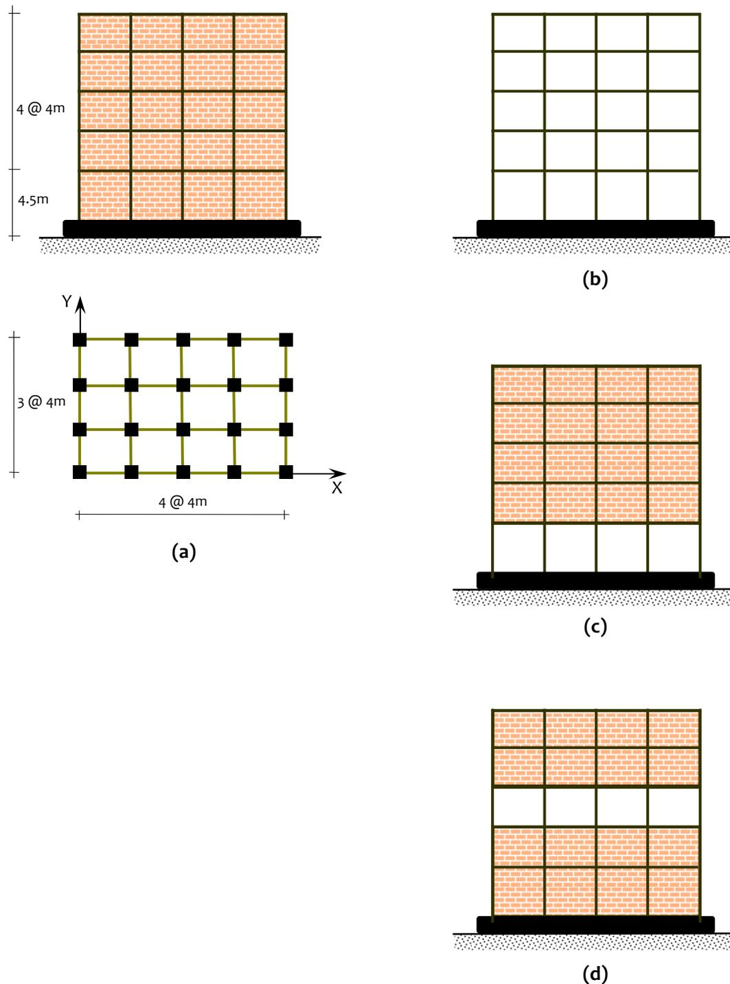
**Figure 4.26:** Open storey in a building: (a) Benchmark 5-storey building with URM infills in all storeys; (b) Bare-frame benchmark 5-storey building with no URM infills in any storey, (c) Similar 5-storey building with URM infills only in upper four storeys, and (d) Similar 5-storey building with URM infills absent in third storey
