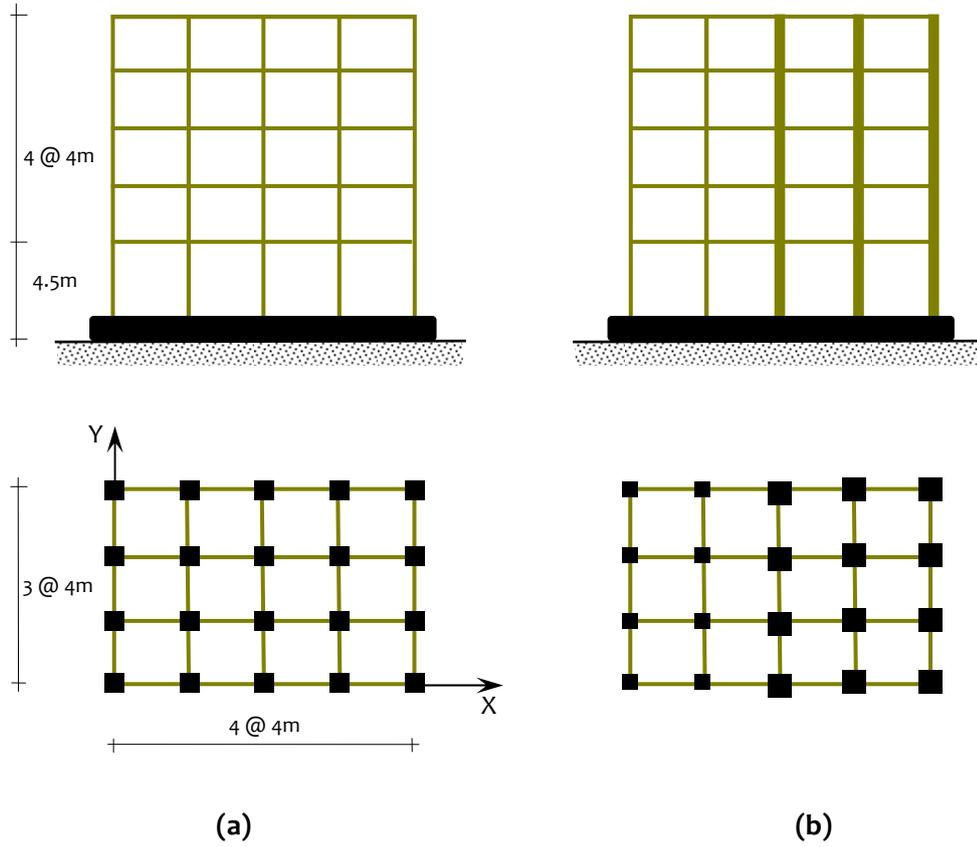
**Figure 4.19:** Lateral strength asymmetry in plan of building: (a) Benchmark 5-storey building with columns of uniform strength; and (b) Similar 5-storey building, but with asymmetry in columns strengths in plan
