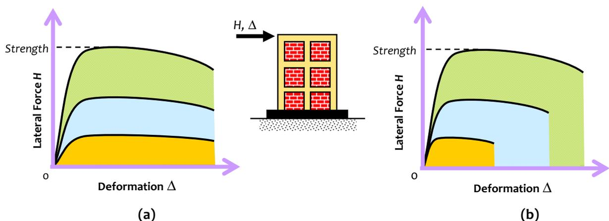
**Figure 4.1:** *Lateral strength of buildings:* Maximum internal resistance offered by buildings under increased displacement loading (a) Buildings having different strengths, but same ductility, and (b) Buildings having different strengths and different ductility
