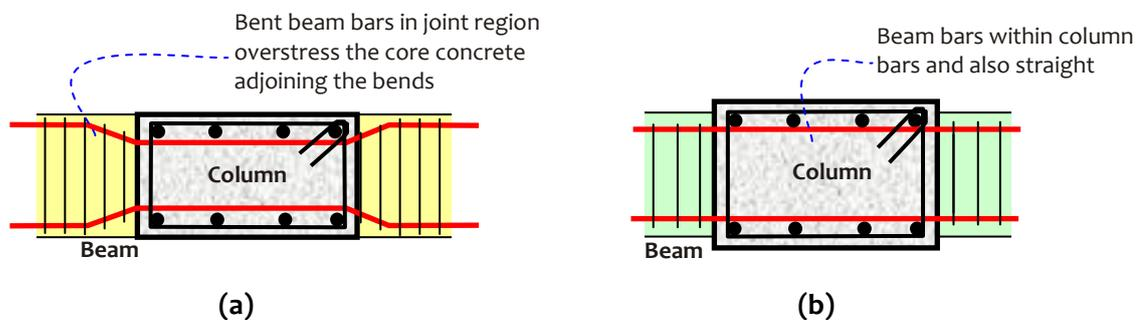
**Figure 4.14:** *Anchorage of beam bars in interior joints:* diagrams show cross-sectional views in plan of joint region - (a) poor practice to bend bars in the joint region, and (b) good practice to use wider column and not bend bars in the joint region
