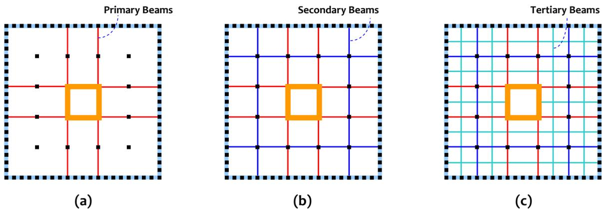
**Figure 3.54:** *Possible systems of beams in a Tube system:* Connection between the core and tube through (a) only *primary* grid of beams, (b) *primary* and *secondary* grid of beams, and (c) *primary*, *secondary* and *tertiary* grid of beams
