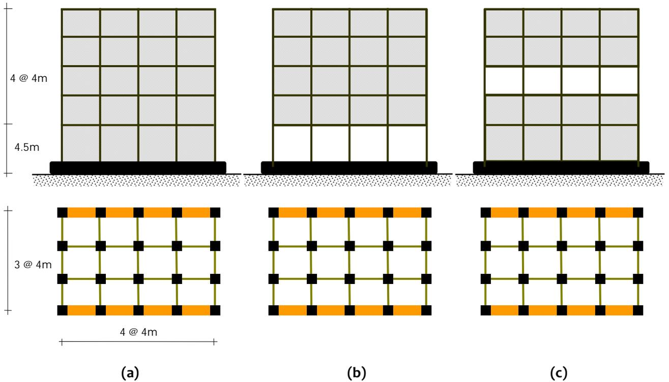
**Figure 4.30:** *Discontinuing Structural Walls in a building: (a) benchmark 5-storey building with Structural Walls in all storeys, (b) similar 5-storey building with Structural Walls discontinued in ground storey; and (c) similar 5-storey building with Structural Walls discontinued in third storey*
