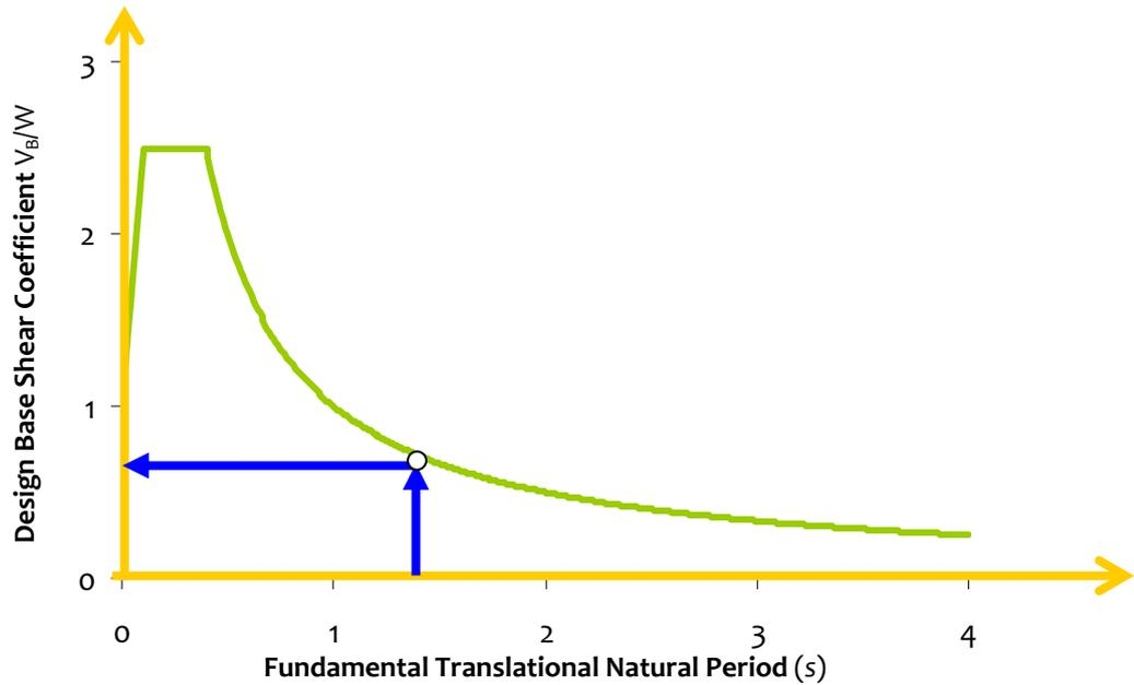
**Figure 2.13:** *Effect of Natural Period on design horizontal seismic force coefficient:* In general, buildings with smaller translational natural period attract higher design seismic force coefficient
