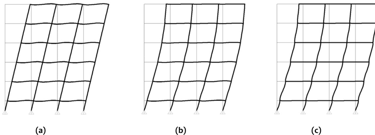
**Figure 2.19:** Effect of relative flexural stiffness of structural elements: Fundamental translational mode shape changes from flexural-type to shear-type with increase in beam flexural stiffness relative to that of column
