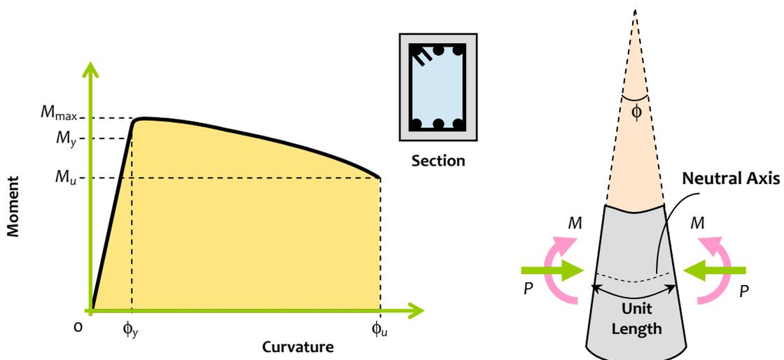
**Figure 4.41:** *Section Ductility:* Typical  $M-\phi$  relationship of an RC member under flexure and axial load
