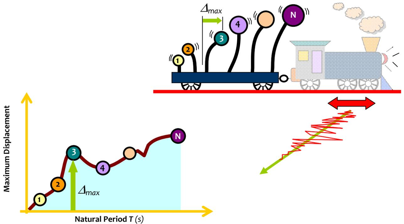
**Figure 2.35:** Influence of same ground motion on buildings with different fundamental translational Natural Period: When the energy content in the earthquake is higher corresponding to the fundamental translational natural period of a building, it shows higher response
