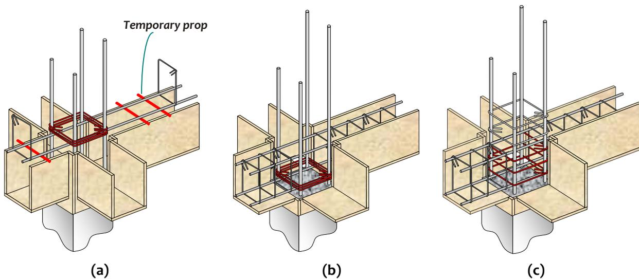
**Figure 4.12:** *Beam-Column Joints in Buildings:* Providing horizontal ties (a) Stage I; (b) Stage II, and (c) Stage III
