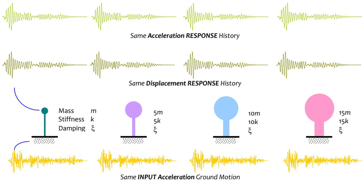
**Figure 2.33:** *Dependence of Response on Natural Period:* Time history of acceleration and displacement of mass is same for a number of structures with same natural period when subjected to the same earthquake shaking, and with same damping
