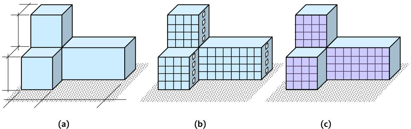
**Figure 1.8:** Components of seismic structural configuration: (a) overall geometry, (b) structural elements (e.g., moment resisting frames and structural walls), and (c) significant non-structural elements (e.g., façade glass)
