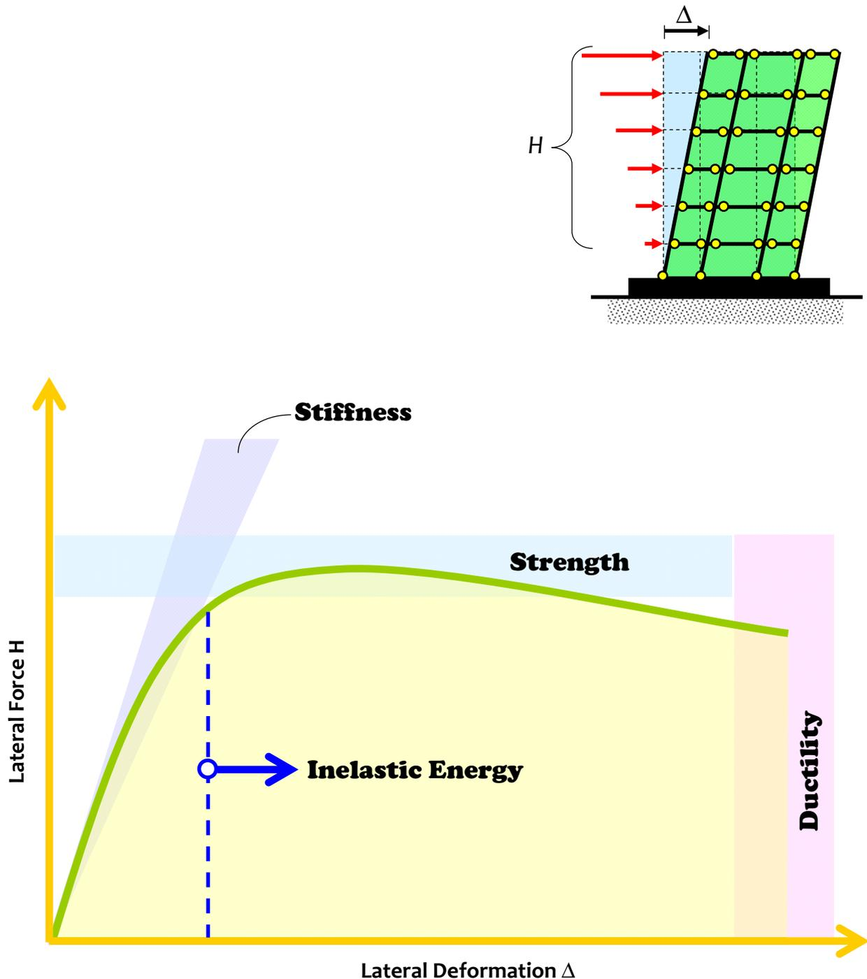
**Figure 5.4:** *Four Virtues of Earthquake-Resistant Buildings* control earthquake performance of buildings: *Stiffness*, *Strength* and *Ductility* directly affect load-deformation behaviour of buildings, while *Seismic Structural Configuration* affects these three virtues indirectly; *Energy Dissipation Capacity* is an overall consequence of all the four virtues of buildings
