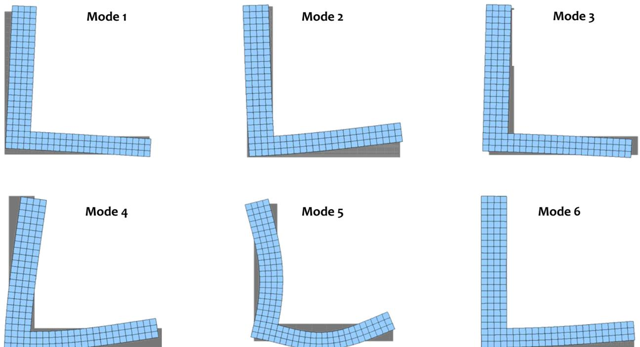
**Figure 3.5:** Modes of oscillation: First six modes of oscillation in building with L-plan shape
