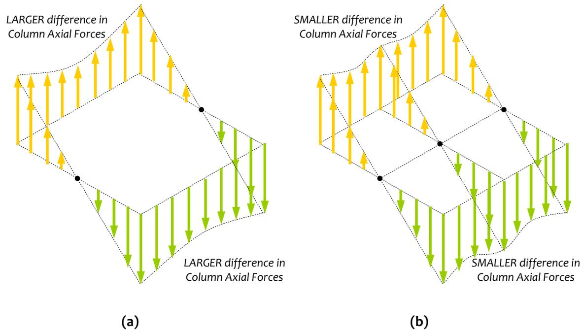
**Figure 3.62:** Shear Lag Effect in Structural Systems: (a) Tube System has large difference in column axial forces on leeward and windward faces, and (b) Tube-in-Tube System has small difference in column axial forces on leeward and windward faces
