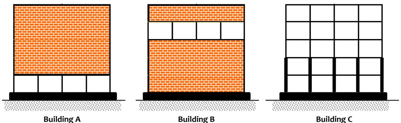
**Figure 3.92:** *Stiffness irregularity in elevation:* Variation of element size and presence of additional or absence of elements in elevation cause overall stiffness irregularity
