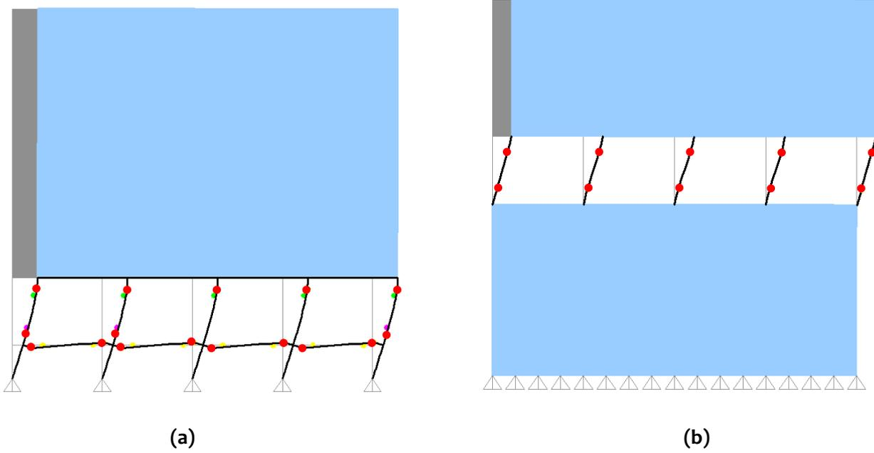
**Figure 4.32:** *Discontinuing Structural Walls in a building:* Open storey attracts the lateral deformation and hence large ductility demand in columns present at that storey, irrespective of the location of the open storey along the height
