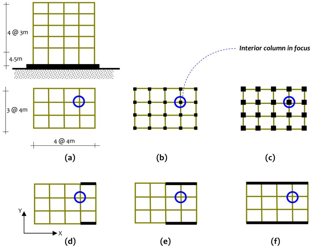
**Figure 4.16:** Strength hierarchy of frame members: (a) benchmark 5-storey building with 400mm×400mm columns; (b) similar 5-storey building with 500mm×500mm columns; (c) similar 5-storey building with 600mm×600mm columns; (d) similar 5-storey building with structural walls in 2 bays; (e) similar 5-storey building with structural walls in 4 bays; (f) similar 5-storey building with structural walls in 8 bays
