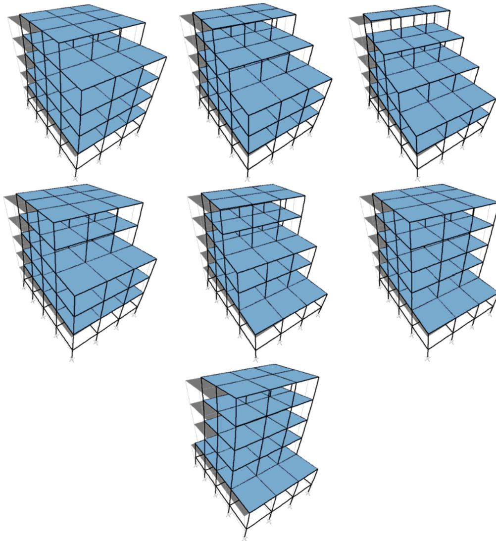
**Figure 3.103:** *Fundamental modes shapes of buildings with vertical irregularity in overall geometry:
