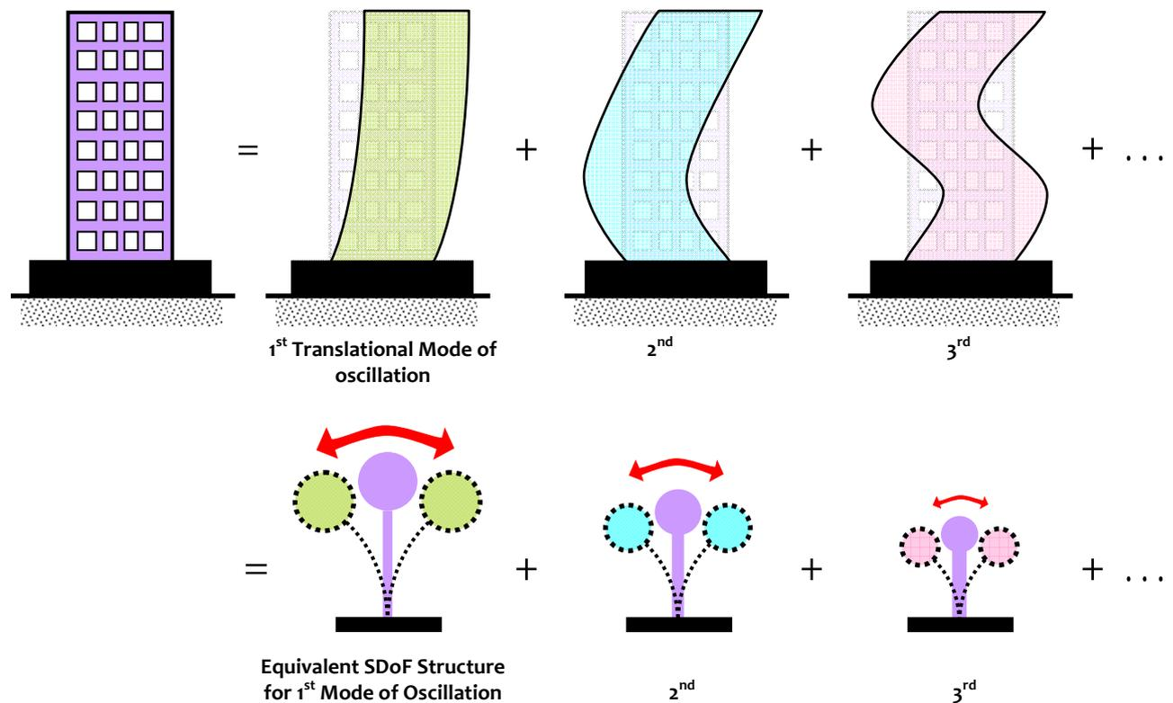
**Figure 2.32:** Equivalent SDoF structures corresponding to each mode of oscillation of the building: Decomposing the response of the building for purposes of understanding behaviour and of undertaking design calculations
