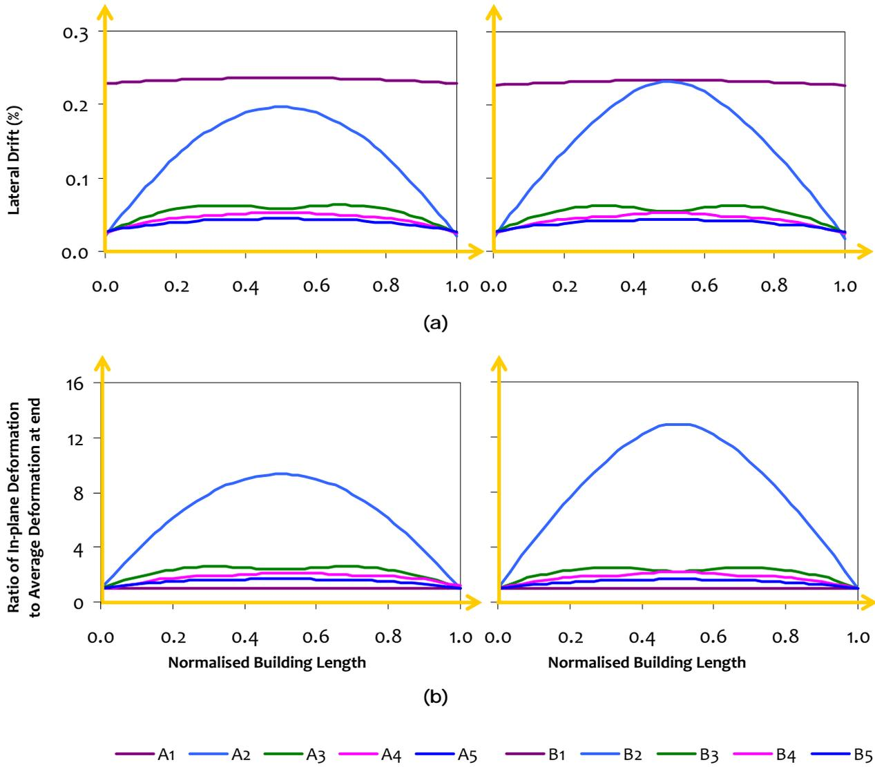
**Figure 3.21:** Roof diaphragm deformation: Cut-outs increase lateral deformation while well distributed LLRS reduces diaphragm flexibility and controls lateral deformation
