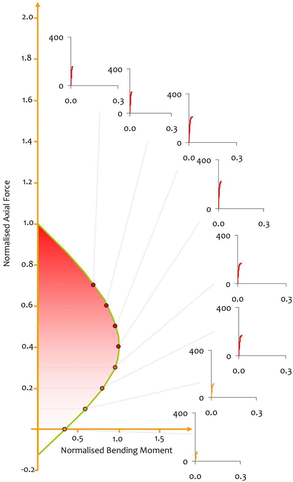
Figure 4.48: DESIGN  $P$ - $M$  interaction envelopes:  $M$ - $\phi$  relations at different axial loads
