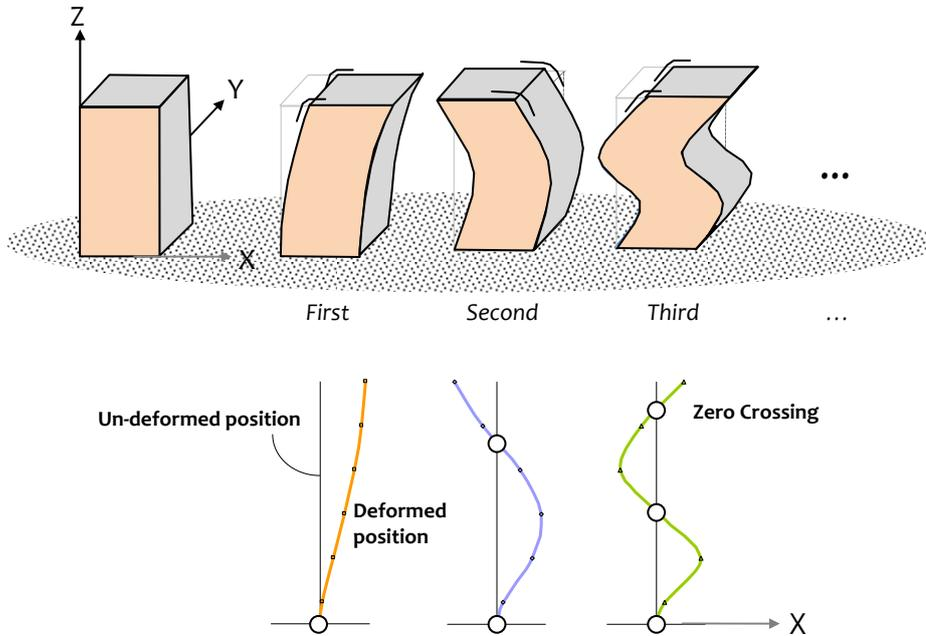
**Figure 2.164:** Fundamental and two higher translational modes of oscillation along X-direction of a five-storey benchmark building: First modes shape has one zero crossing of the un-deformed position, second two, and third three
