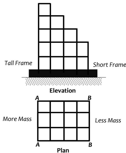
**Figure 3.101:** Characteristics of buildings with vertical irregularity in overall geometry: Step-back buildings have frames of different heights, leading to unsymmetrical stiffness and mass distributions in plan
