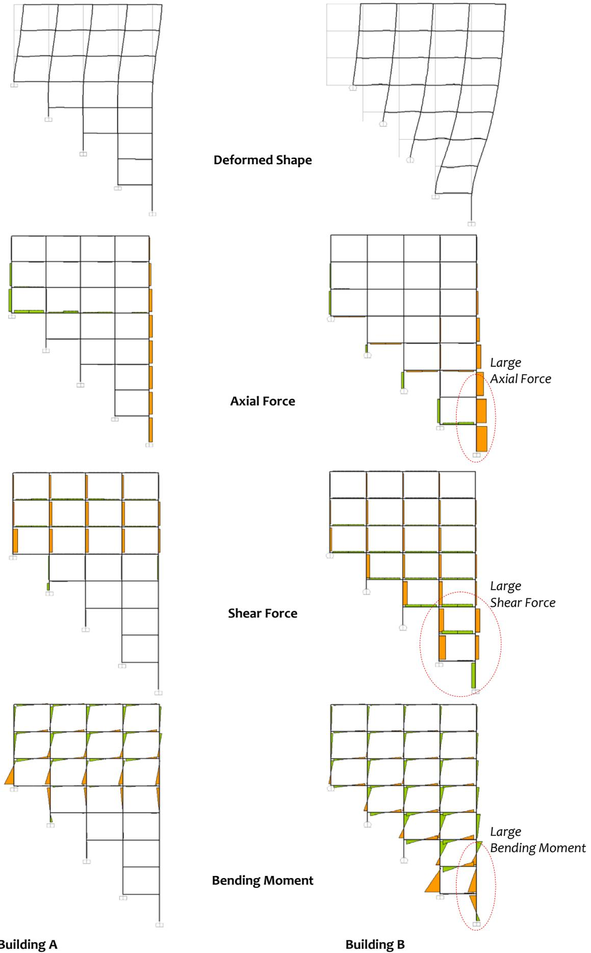
Figure 3.99: Buildings on slope: Deformation and force distribution
