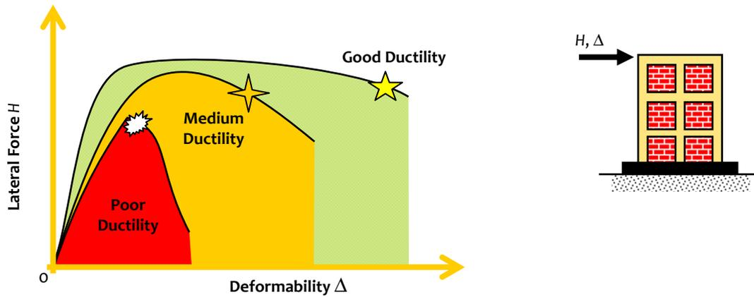
**Figure 4.39:** Energy absorption owing to ductility: Three structures possess different levels of ductility, and hence different energy absorption capacities
