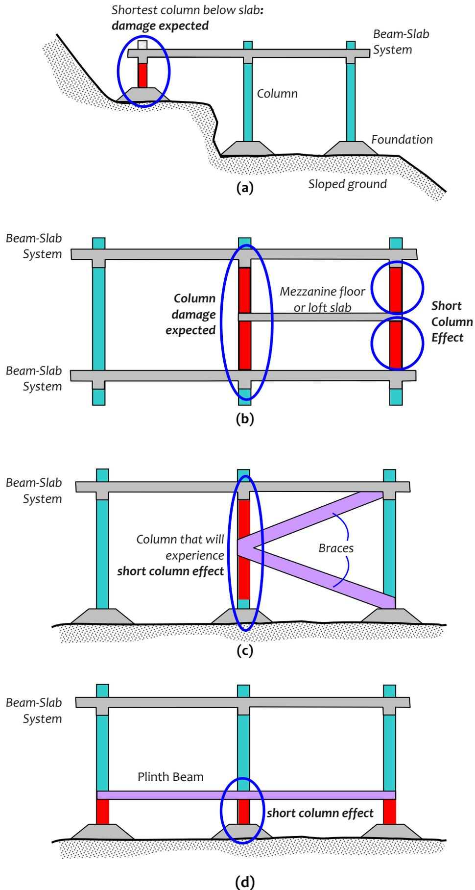
**Figure 4.34:** Short column effect owing to other causes in RC columns in buildings: Damages in restricted areas in columns (a) sloping ground, (b) mezzanine slab, (c) staircase beam/slab or K-braces on building columns, and (d) use of plinth beams in ground storey
