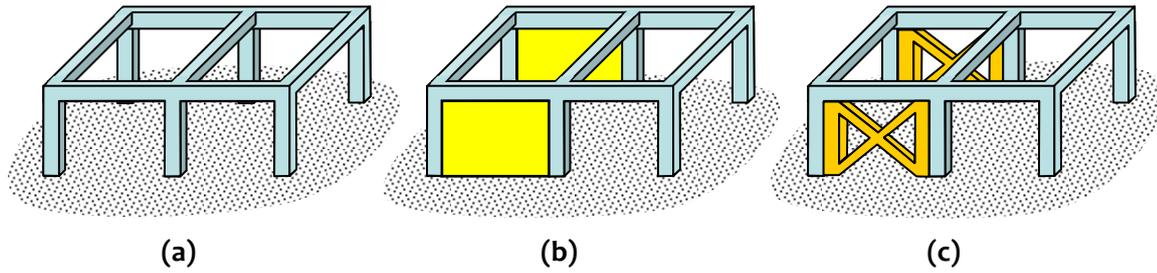
**Figure 3.29:** Common structural systems employed in buildings: (a) Moment frames, (b) Moment frames with structural walls, and (c) Braced moment frames. Walls and braces shown are shown only along one direction in plan; but designers can choose to provide them along both directions.
