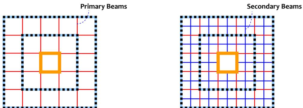
**Figure 3.59:** *Beams in Tube-in-Tube Systems:* Secondary beams help in transferring the gravity loads to the two tubes and the core
