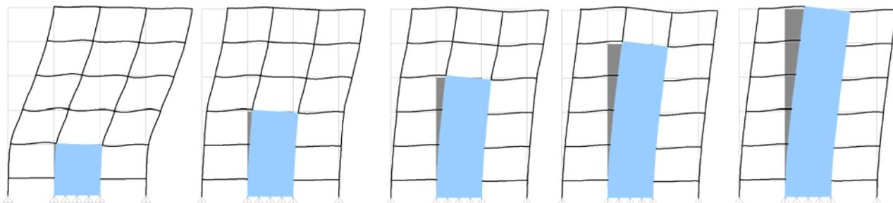
**Figure 3.78:** *Discontinuing structural wall in upper storeys:* Large deformation demand in storey immediately above structural wall
