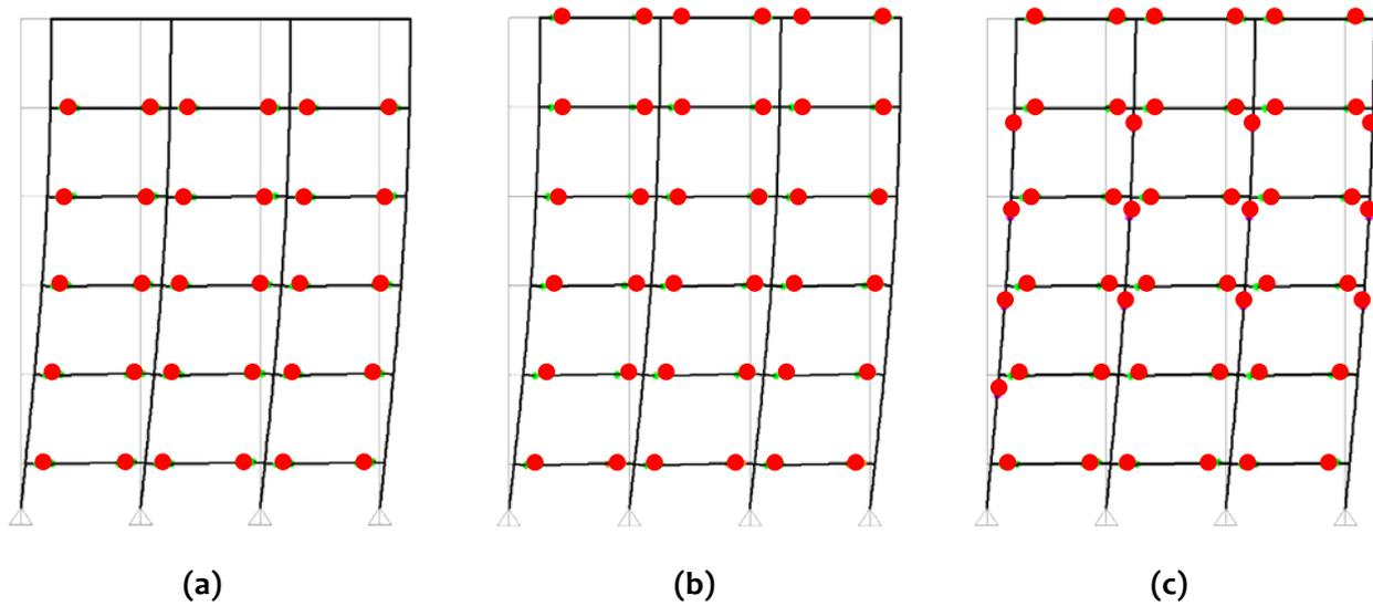
**Figure 4.21:** *Lateral strength asymmetry in plan of building:* Strength-asymmetric buildings attract more demand on stronger columns and undergo undesirable column inelasticity - (a) frame in benchmark building with damage in *beams*, (b) strength asymmetry building frames with weaker columns sustain damage in *beams*, and (c) strength asymmetry building frames with stronger columns sustain damage in *columns*
