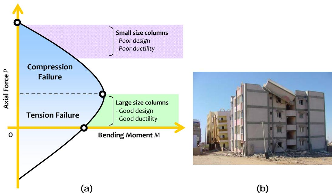
**Figure 4.8:** Sizing of columns in buildings: (a) Schematic of  $P$ - $M$  Interaction diagram of RC columns, and (b) All buildings on a street lost their open ground storey during 2001 Bhuj Earthquake (India); they had small size columns (*i.e.*, 230 mm wide, 450 mm long)
